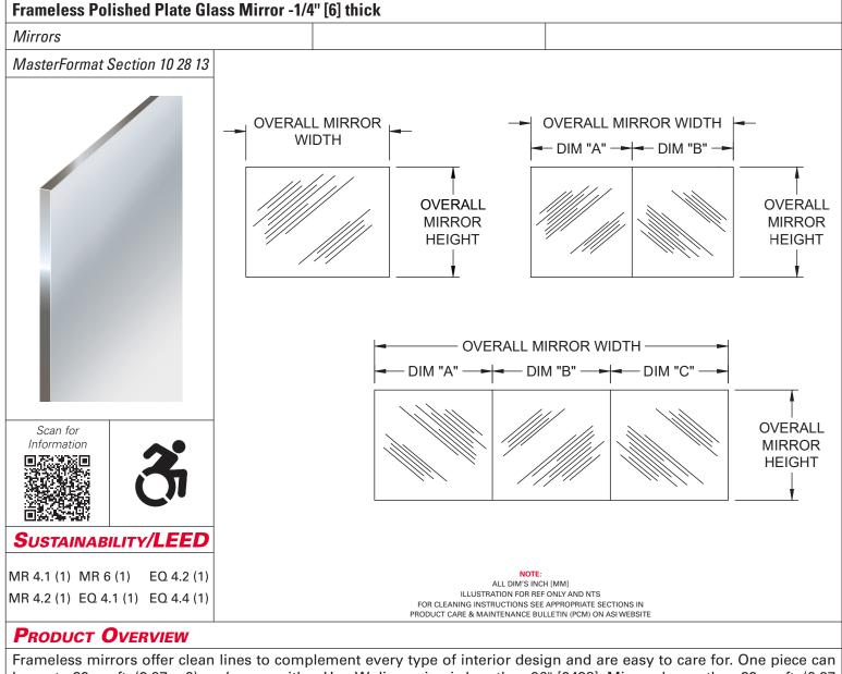
be up to 32 sq. ft. (2.97 m2), as long as either H or W dimension is less than 96" [2438]. Mirrors larger than 32 sq. ft. (2.97 m2) or with either linear H or W dimension larger than 96" [2438] shall be supplied as multiple pieces. Made of 1/4" [6] polished plate glass.
