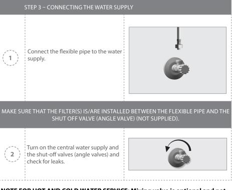
NOTE FOR HOT AND COLD WATER SERVICE: Mixing valve is optional and not supplied by ASI, may be supplied by others, and will require hot & cold potable water building service (by others).
